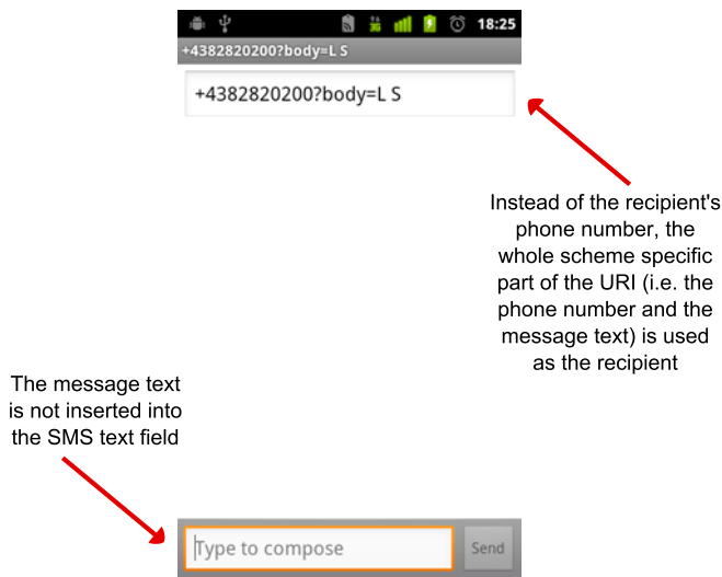
Fig. 3. On Android 2.3.4, the URI triggers the messaging application. This application extracts the whole scheme-specific part of the URI, "+4382820200?body=L%20S", and uses this as the recipient's phone number. The message text remains empty.
